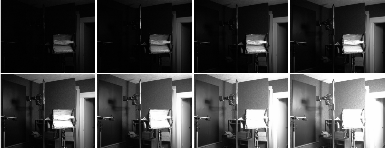
Figure 1: Eight pictures of a static scene taken at different exposure times. The camera used was a Nikon E2N, and the image resolution is 640 \times 500 . The exposure times are (a) 1/1000 sec. (b) 1/500 sec. (c) 1/250 sec. (d) 1/125 sec. (e) 1/60 sec. (f) 1/30 sec. (g) 1/15 sec. (h) 1/8 sec.
