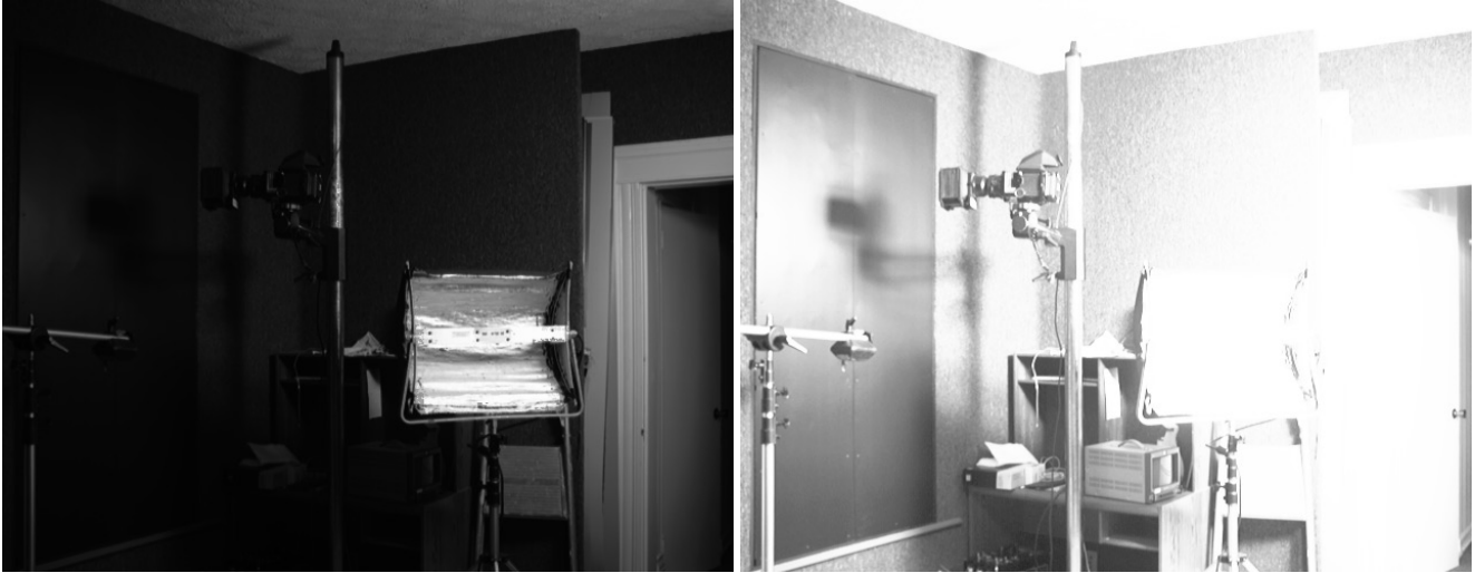
Figure 4: a b High dynamic range output images. (a) Full dynamic range mapped to eight bits; (b) using high dynamic range image data to simulate camera output for an exposure time of 1/3 sec.
